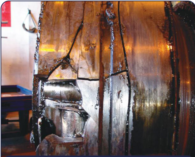
The damage to the bearing was very noticeable and consistent with the sound file pattern
