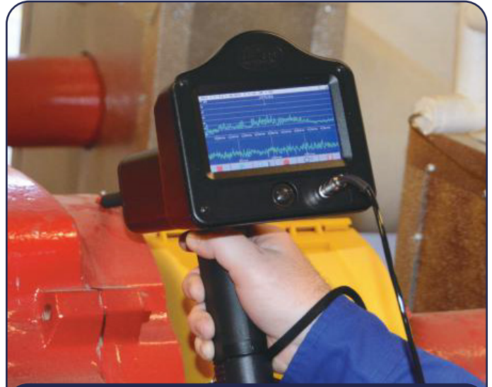
Ultrasound instrument with sound recording is the perfect tool to monitor the condition of slow speed bearings.
